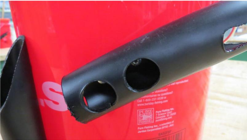
**Place rod holder 4 inches from bottom of bucket at a 30 degree angle. Attach the pipe to the bucket using bolts or rivets. Drill  $\frac{3}{16}$ <sup>th</sup> inch holes in rod holder though the  $\frac{1}{2}$ " inch holes and into bucket (use  $\frac{3}{16}$ 's rivet or  $\frac{1}{8}$ <sup>th</sup> inch bolts with 2 washers) The head of rivet or bolt should be on the outside of bucket (nuts or nipple of rivet should be on inside bucket).**
