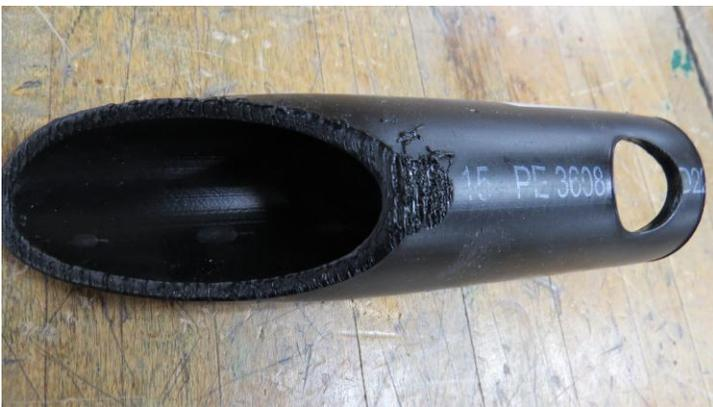
**On 2 pipes, drill one 1/2inch hole on the angled side (not pointed side)
