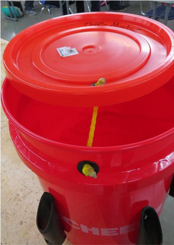
**Drill hole in lid 1 inch from lid edge. Thread rope into holes with end of rope toward outside of bucket and lid. Tie simple knot on both ends.**
