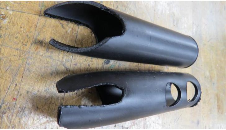
**On the 3<sup>rd</sup> pipe, two holes are needed on opposite sides toward lower end of pipe. (Spacing is one finger width from bottom and one finger width to the next hole) On opposite side of angle cut  $\frac{1}{2}$ " groove down 2 inches.**
